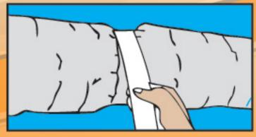
Pull jacket and insulation back over the core. Use atleast 2 wraps of duct tap to tape the jacket.
