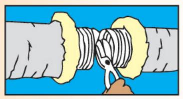
Cut completely around and through the duct with knife or scissors. Cut the wire with cutters. Fold back the jacket and insulation.
