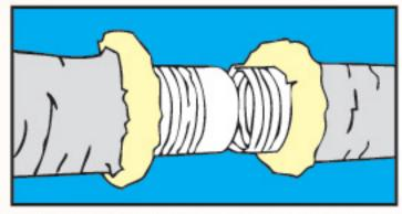
Fold back jacket and insulation from core. Butt 2 cores together on a standard 4" (100mm) length metel sleeve.
