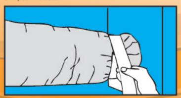
Pull jacket and insulation back over the core. Use atleast 2 wraps of duct tap to tape the jacket. You may use a clamp along with or instead of the duct tape.
